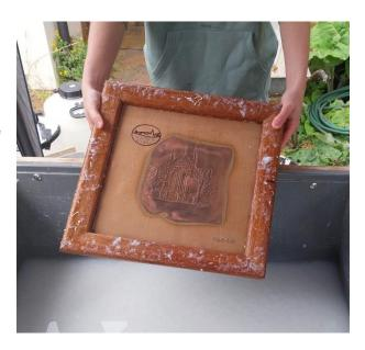
The papermaking stock, the pulp, in the case of the demonstration was cotton linters suspended in water. Linters is the fine fuzz of very short cotton fibres left on the cotton seed
